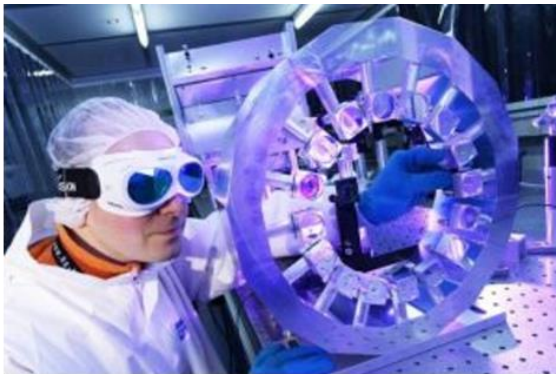
Multipass thin disk Yb:YAG amplifier part of a DPSSL developed at the MBI
