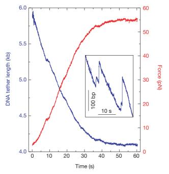
**Figure 2** Measurements of packaging in no feedback mode. The tether shortens (blue line) and the force increases (red line) as the portal motor pulls in the DNA. In this example, the motor stalled at a force of  $\sim$ 55 pN. Although in many measurements the linkage broke before stalling was observed, similar maximum forces could be projected from
