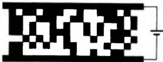
Fig. 24. Definition of the conductance of a random conductor network. All copper squares in the topmost row of the lattice are connected to a heavy copper bar (no loss of energy in the bar), and so are all squares in the bottom row. A battery then applies a unit voltage between these two bars. The resulting electrical current is called the conductance.
