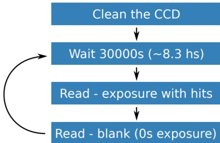
The blank images provide an excellent measurement of the background produced by readout noise
