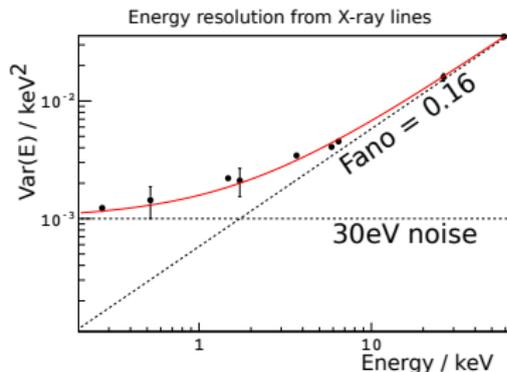
**Electron energy scale calibrated down to 280eV, 63eV RMS @6keV**
