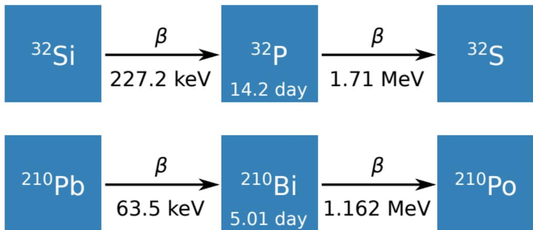
Low energy electrons from  $\beta$  decays could be a significant background in silicon
