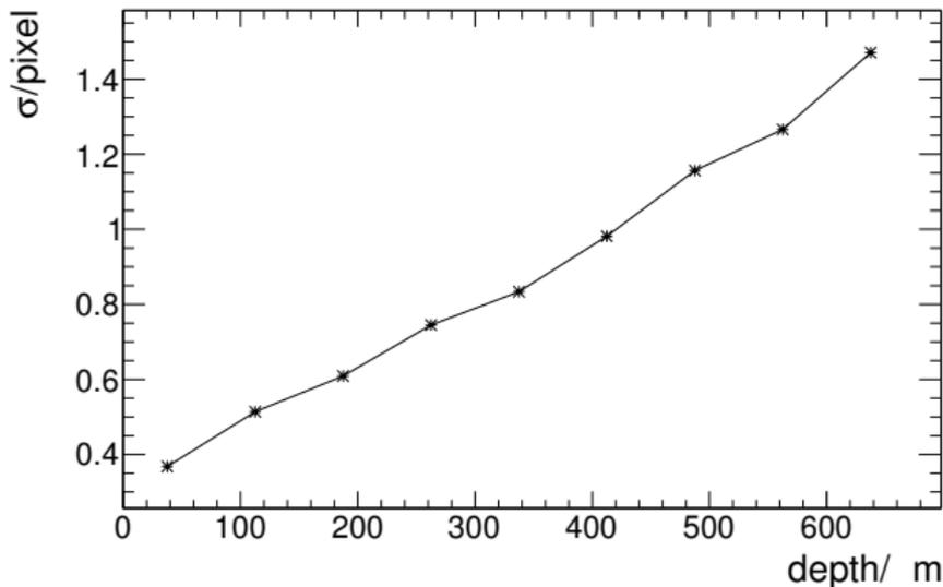
Diffusion can be measured as a function of the interaction depth.
