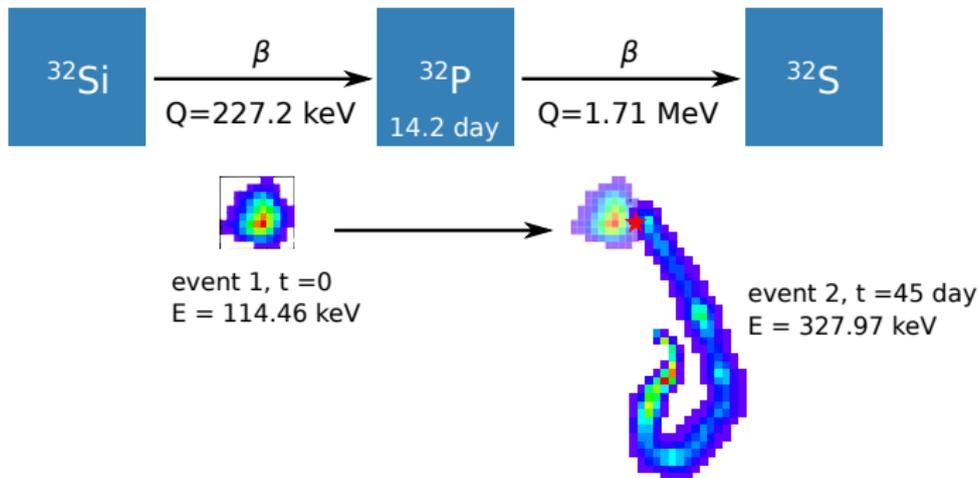
The pixilation of the DAMIC detector allows us reject this background.
