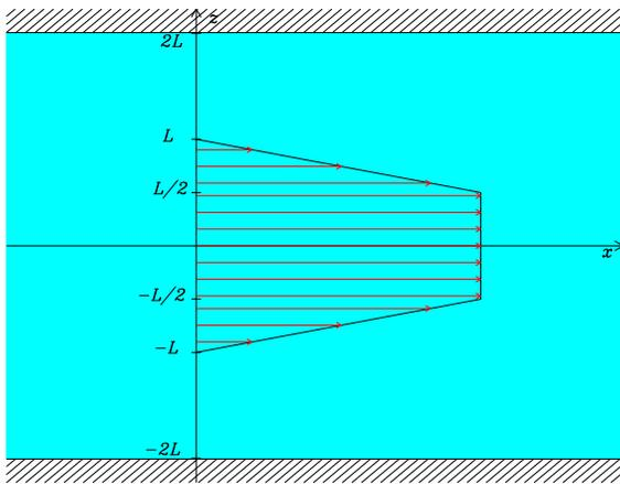
$$U(z) = \begin{cases} 0 & \text{si } L \leq z \leq 2L \\ \frac{2U_0}{L}(L - z) & \text{si } L/2 \leq z \leq L \\ U_0 & \text{si } -L/2 \leq z \leq L/2 \\ \frac{2U_0}{L}(L + z) & \text{si } -L \leq z \leq -L/2 \\ 0 & \text{si } -2L \leq z \leq -L \end{cases} .$$
