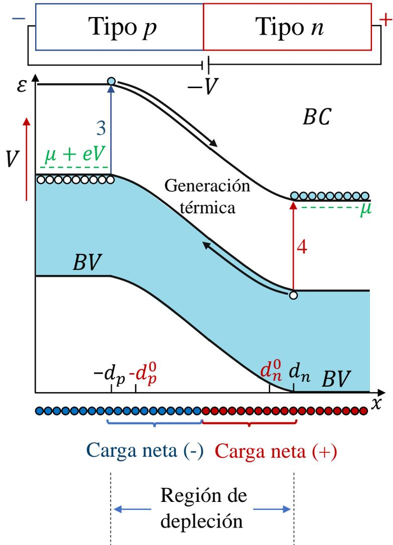
$$j = en_i^2 \left( \frac{D_n}{L_n N_a} + \frac{D_p}{L_p N_d} \right) \left( e^{\frac{V}{k_B T}} - 1 \right) = en_i^2 \left( \frac{L_n}{N_a \tau_n} + \frac{L_p}{N_d \tau_p} \right) \left( e^{\frac{V}{k_B T}} - 1 \right)$$
