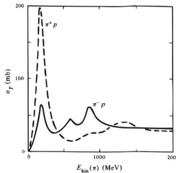
Figure 5.35: Total cross section as a function of pion kinetic energy for the scattering of positive and negative pions from protons. (1 mb = 1 millibarn =  $10^{-27}$  cm<sup>2</sup>.)
