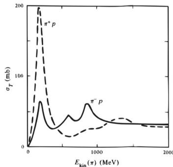
Figure 5.35: Total cross section as a function of pion kinetic energy for the scattering of positive and negative pions from protons. (1 mb = 1 millibarn =  $10^{-27}$  cm<sup>2</sup>.)
