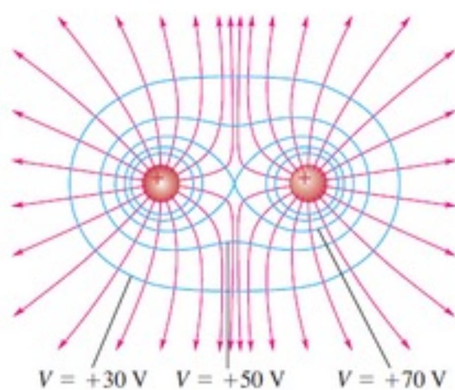
➔ Electric field lines      — Cross sections of equipotential surfaces
