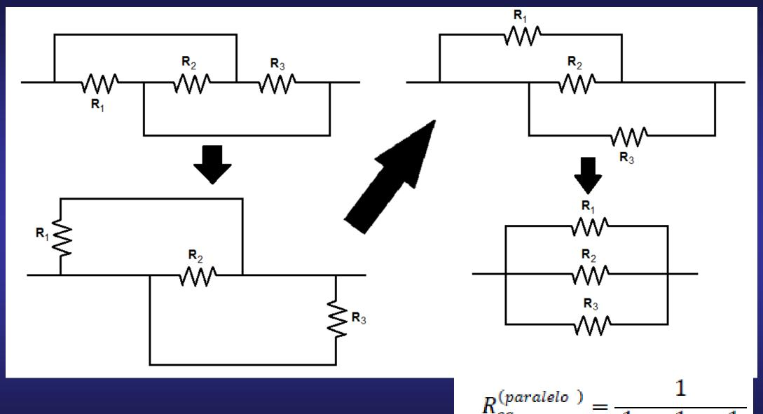
$$R_{eq}^{(paralelo\ )} = \frac{1}{\frac{1}{R_1} + \frac{1}{R_2} + \frac{1}{R_3}}$$
