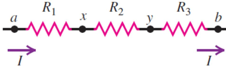
$$V_{ax} = IR_1 \quad V_{xy} = IR_2 \quad V_{yb} = IR_3$$
