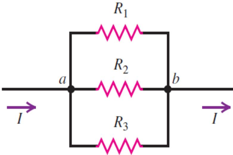
$$I_1 = \frac{V_{ab}}{R_1} \quad I_2 = \frac{V_{ab}}{R_2} \quad I_3 = \frac{V_{ab}}{R_3}$$
