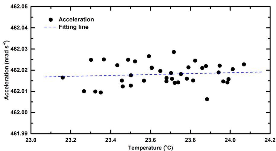
**Extended Data Fig. 4 | Effect of temperature on the measurement of the angular acceleration in the AAF method.** A modulation experiment was carried out by increasing the temperature variation in the room to about 1 °C. Solid circles represent the average angular acceleration of the pendulum turntable over 12-h data taking periods. The dashed line with
