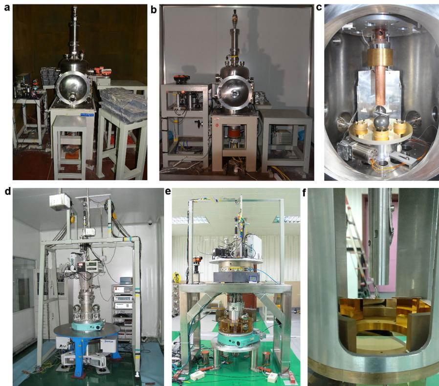
**Extended Data Fig. 1 | Photographs of the experimental apparatus.** **a**, Apparatus 1, used in TOS-I. **b**, Apparatus 2, used in TOS-II. **c**, The suspended pendulum and source masses in the vacuum chamber used in the TOS method. The copper tube around the fibre is used to reduce the temperature gradient. The electrostatic shield (here elevated to show the pendulum), the three-point mounts, the ULE-glass disk and the
