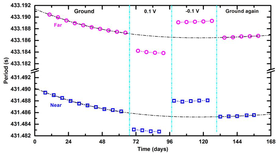
**Extended Data Fig. 5 | Electrostatic effect on the measurement of the pendulum period in the TOS method.** Different voltages are applied on the shield in the sequence: ground, 0.1 V, -0.1 V, ground. For each voltage, 4–5 sets of measurements of the pendulum period are performed at the ‘near’ and ‘far’ configurations. The corresponding change of the frequency squared ( $\Delta\omega^2$ ) for the steps of the sequence is determined to be
