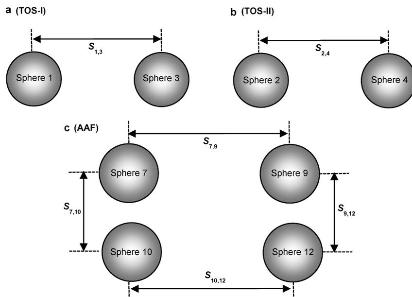
**Extended Data Fig. 3 | Schematic diagram of the source masses.** **a, b,** In the TOS method, spheres 1 and 3 are used in apparatus 1 (TOS-I; **a**) and spheres 2 and 4 are used in apparatus 2 (TOS-II; **b**).  $S_{1,3}$  and  $S_{2,4}$  are the horizontal distances of the geometric centres of the spheres in apparatus
