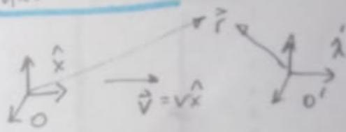
$$\left. \begin{array}{l} \vec{r} = (x, y, z) \\ x' = x - vt \\ y' = y \\ z' = z \\ t' = t \end{array} \right\}$$
