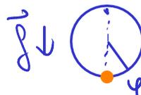
$$\varphi_{eq}^{(3)} = \arccos\left(\frac{g}{\omega^2 R}\right) \quad * \quad \cos\left[\arccos\left(\frac{g}{\omega^2 R}\right)\right] = \frac{g}{\omega^2 R}$$
