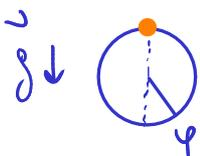
$\varphi_{eq}^{(1)} = 0 \Rightarrow \frac{dF}{d\varphi}(\varphi_{eq} = 0) = -mg + m\omega^2 R$
