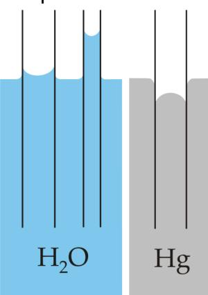
Capillary action is the result of adhesion and surface tension. Adhesion of water to the walls of a vessel will cause an upward force on the liquid at the edges and result in a meniscus which turns upward. The surface tension acts to hold the surface intact, so instead of just the edges moving upward, the whole liquid surface is dragged upward.
