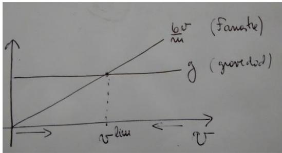
$$\frac{dv}{dt} = \overset{\text{aumento}}{\tilde{g}} - \overset{\text{disminución}}{\frac{b}{m}v}$$
