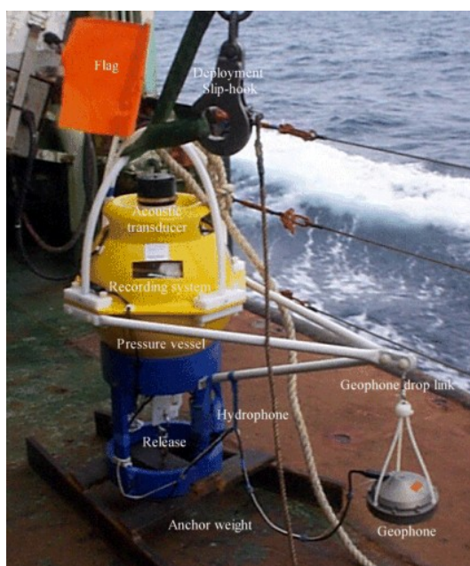
Figure 6. Different parts of the OBS preliminary design using glass sphere. Hydrophone detail from Hytech Company.
