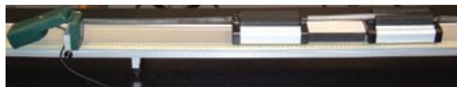
Fig. 1. Equipment setup. Note that excessive displacement in the oscillation may cause a separation between the wood friction block and the carts.
