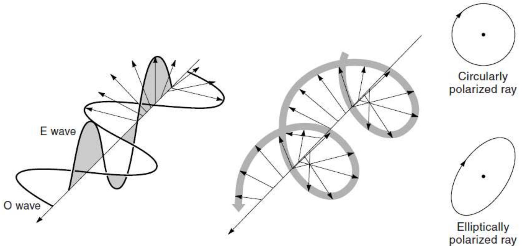
The waveforms of elliptically and circularly polarized light. O and E rays following the same propagation axis but vibrating in mutually perpendicular planes cannot interfere, but can be combined by vector addition. Depending on the relative phase difference between the two rays, the resultant wave may be linear or take on the form of a spiraling ellipse or circle. With a phase displacement of  $\pi/4$ , the waveform is a circle.
