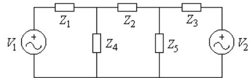
Datos:  $V_1 = 30\text{V}$ ,  $V_2 = 20\text{ V}$ ,  $Z_1 = 5\ \Omega$ ,  $Z_2 = 4\ \Omega$ ,  $Z_3 = (2+3j)\ \Omega$ ,  $Z_4 = 5j\ \Omega$ ,  $Z_5 = 6\ \Omega$  y  $f = 50\text{Hz}$ .
