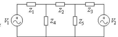
Datos:  $V_1 = 30\text{ V}$ ,  $V_2 = 20\text{ V}$ ,  $Z_1 = 5\ \Omega$ ,  $Z_2 = 4\ \Omega$ ,  $Z_3 = (2 + 3j)\ \Omega$ ,  $Z_4 = 5i\ \Omega$ ,  $Z_5 = 6\ \Omega$  y  $f = 50\text{ Hz}$ .
