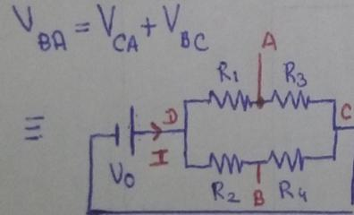
$V_{CD} = -V_0$ ;  $I_A = \frac{V_{CD}}{R_1 + R_3} = \frac{-V_0}{R_1 + R_3}$
