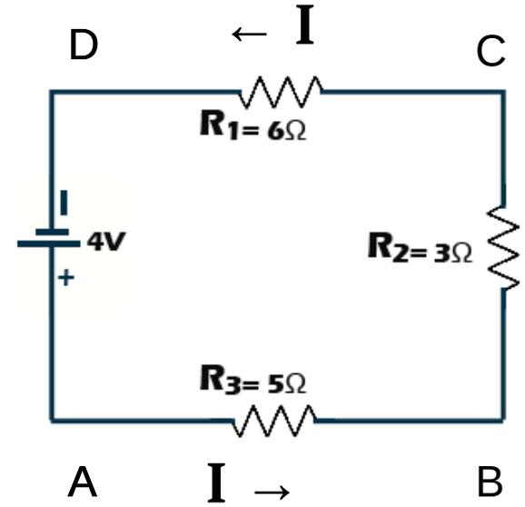
$$\begin{aligned} 0 &= V_{AA} = V_{BA} + V_{CB} + V_{DC} + V_{AD} = -I \cdot R_3 - I \cdot R_2 - I \cdot R_1 + \text{fem} = -I(R_1 + R_2 + R_3) + 4V = \\ &= -I R_{\text{equiv}} + 4V \rightarrow I = 4V / R_{\text{equiv}} \rightarrow I = 0.28A \end{aligned}$$
