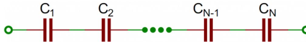
$$\frac{1}{C_{Tot}} = \frac{1}{C_1} + \frac{1}{C_2} + \dots + \frac{1}{C_{N-1}} + \frac{1}{C_N}$$
