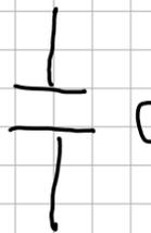
$\rightarrow Z_C = \frac{1}{i\omega C} = \frac{-i}{\omega C} = \frac{e^{-i\pi/2}}{\omega C}$  cambia la fase
