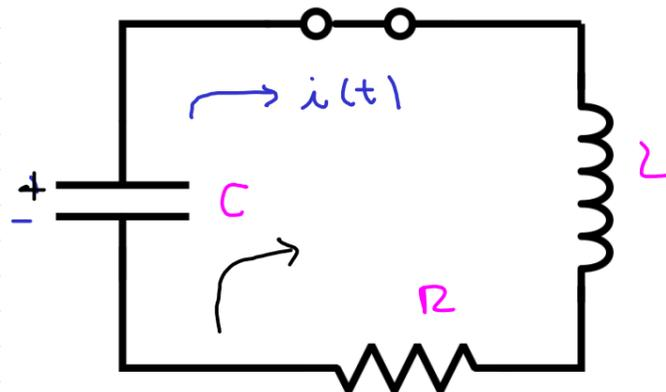
$$\frac{q}{C} - iR - L \frac{di}{dt} = 0 \quad \longrightarrow \quad \frac{q}{C} + \frac{dq}{dt} R + L \frac{d^2 q}{dt^2} = 0$$
