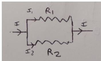
$$\text{Si } R_1 = R_2 = R \Rightarrow R_{eq} = \frac{R}{2}$$
