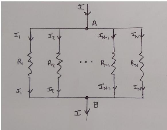
$$V(A) - V(B) = I_1 R_1 = I_2 R_2 = I_3 R_3 = \dots = I_N R_N \Rightarrow I_k = \frac{V(A) - V(B)}{R_k}$$
