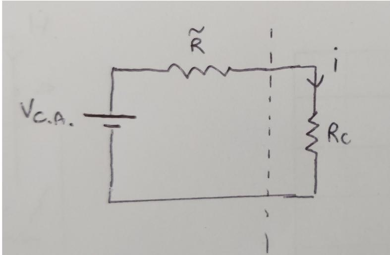
$$V_{c.a.} = i(\tilde{R} + R_c) \Rightarrow i = \frac{V_{c.a.}}{R_c + \tilde{R}}$$
