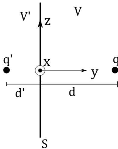
$$\phi(\vec{r}) = \frac{kq'}{|\vec{r} - (-d')\hat{y}|} + \frac{kq}{|\vec{r} - d\hat{y}|} \quad , \quad \phi(x, 0, z) = 0$$
