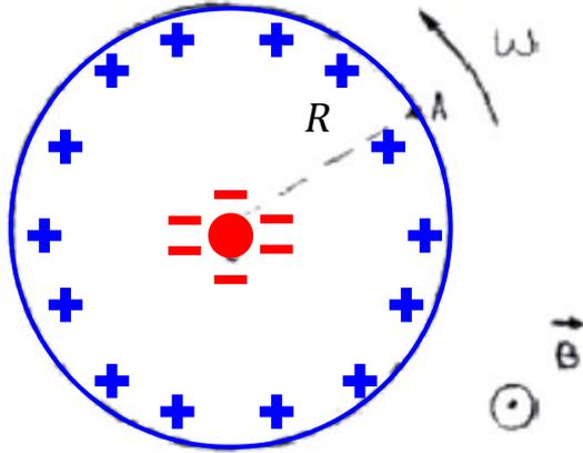
$$\vec{F} = q(\vec{E} + \vec{v} \times \vec{B}) = 0 \implies \vec{E} = -\vec{v} \times \vec{B}$$
