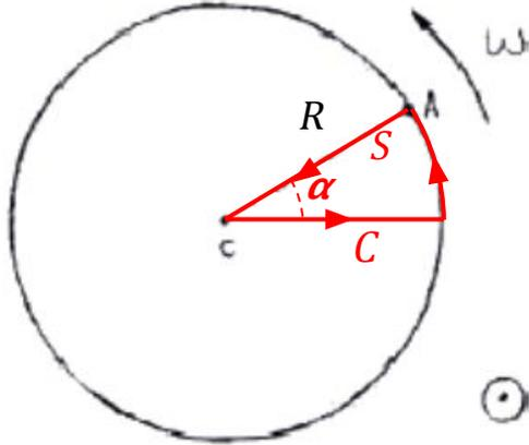
$$A(t) = \frac{R^2}{2}\alpha(t) = \frac{R^2}{2}\omega t \quad \hat{n} = \hat{z} \quad \bar{B} = \bar{B}_0\hat{z}$$
