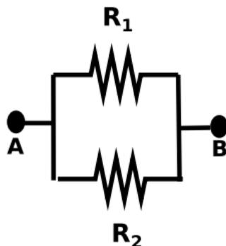
$$R_{\text{eq}}^{AB} = \left( \frac{1}{R_1} + \frac{1}{R_2} \right)^{-1}$$
