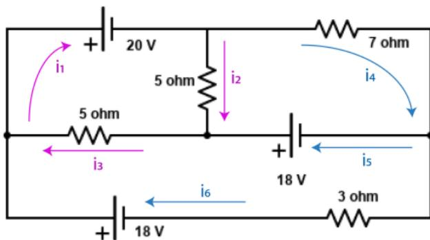
$$\Delta V_{CD} = V_C - V_D = 18V - i_3 5\Omega = \frac{1053}{46}V$$
