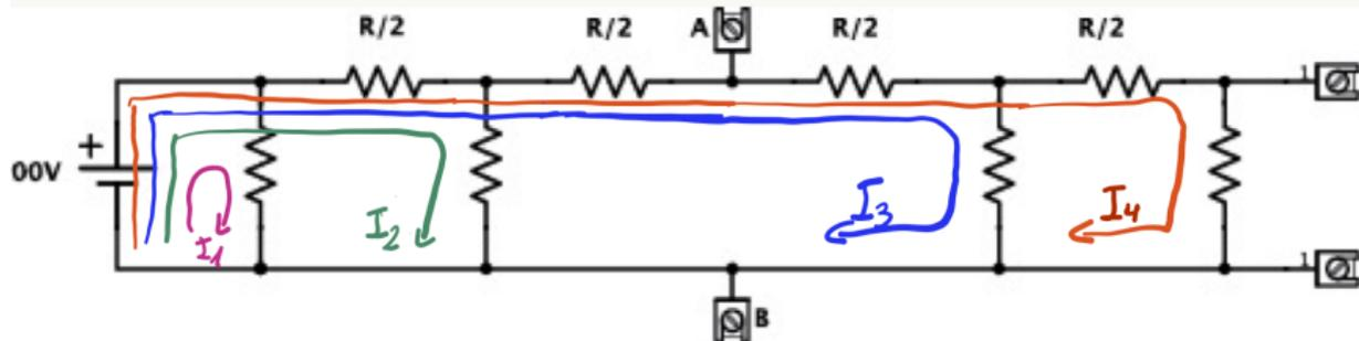
$$\begin{aligned}V_{eq}^{AB} &= (I_3 + I_4) \frac{R}{2} - I_2 R \\&= 2I_3 \frac{R}{2} - I_2 R \\&= \frac{2}{11} \frac{V}{R} R - \frac{6}{11} \frac{V}{R} R \\&= -\frac{4}{11} V = -\frac{400}{11} \text{ Volt}\end{aligned}$$
