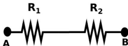
$$R_{\text{eq}}^{AB} = R_1 + R_2$$
