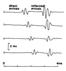
Fig. 8. Typical waveforms obtained for z = 0.4 m and x values of 0.4, 0.5, 0.6, and 0.7 m. The earlier arrivals are the direct wave and the later arrivals are the reflected wave.
