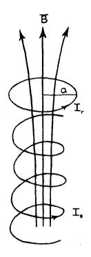
Fig. 3. Schematic of Thomson's jumping ring, placed somewhat above a concentric solenoid.
