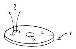
Fig. 4. Schematic of an eddy current brake, with a disk of radius a spinning about a vertical, with the axis in a fixed vertical **B** field confined to a square region of side b.
