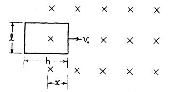
Fig. 1. A current loop of resistance R, inductance L, and mass M moving into a fixed magnetic field B.
