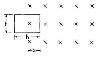
Fig. 2. A current loop partially in an oscillating magnetic field B.
