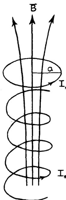
Fig. 3. Schematic of Thomson's jumping ring, placed somewhat above a concentric solenoid.
