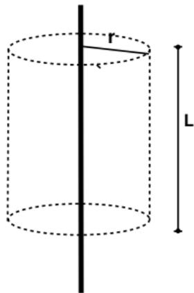
$$\int \int E(r) \hat{r} \cdot d\vec{S} = \int \int_{\text{TAPA}_{\text{SUP}}} E(r) \hat{r} \cdot \hat{z} r dr d\phi + \int \int_{\text{TAPA}_{\text{INF}}} E(r) \hat{r} \cdot (-\hat{z}) r dr d\phi + \int \int_{\text{PARED}} E(r) \hat{r} \cdot \hat{r} r dz d\phi$$
