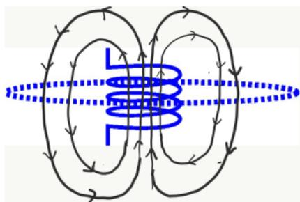
$$M_{12} = \frac{\Phi_{12}}{I_2} = \frac{\int \int_{S_{\text{sol}}} \vec{B}_{\text{esp.}} \cdot d\vec{S}_{\text{sol}}}{I_2} = \frac{\mu_0 \pi R_1^2 N_1}{2\sqrt{L^2/4 + R_2^2}}$$
