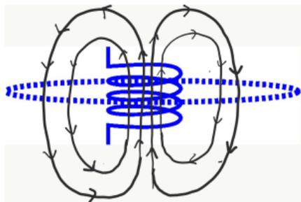
$$M_{12} = \frac{\Phi_{12}}{I_2} = \frac{\int \int_{S_{sol}} \vec{B}_{esp} \cdot d\vec{S}_{sol}}{I_2} = \frac{\mu_0 \pi R_1^2 N_1}{2\sqrt{L^2/4 + R_2^2}}$$
