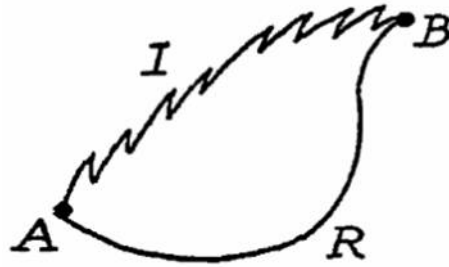
Figure 4.3: A reversible path R from A to B and an irreversible path I from B to A.
