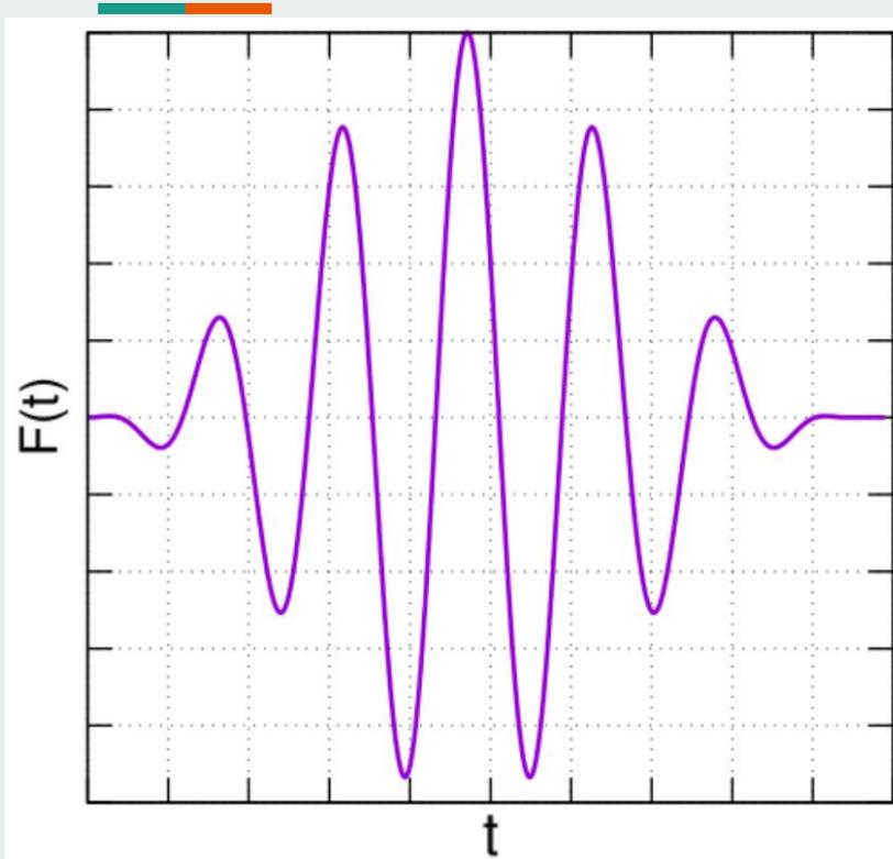
$$F(t) = \begin{cases} \overbrace{F_0 \sin(\omega_p t + \phi)}^{\text{Portadora}} \overbrace{\sin^2(\pi t / \tau)}^{\text{Envolvente}} & 0 \leq t \leq \tau \\ 0 & t > \tau, \end{cases}$$
