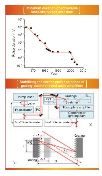
The mJ-level, sub-10-fs laser pulses needed to create atto-second pulses are generated by chirped pulse amplifiers (CPA), as shown in part (a) of the lower figure on this page, followed by hollow-core fiber compressors. CEP control usually begins in the femtosecond oscillators. The oscillator output is a pulse train that corresponds to a comb of longitudinal modes in the frequency domain.
