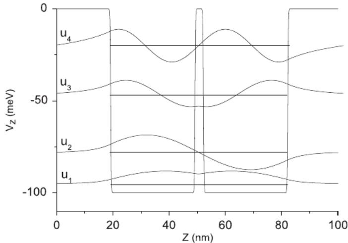
**Fig. 1.** The  $\text{Al}_{0.1}\text{In}_{0.9}\text{Sb}$ - $\text{InSb}$  double-well confining potential in the longitudinal direction of the quasi-one-dimensional nanowhisker quantum dots. The single-particle eigenfunctions and energies are also shown.
