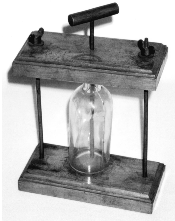
Bottle Bursting Apparatus. This apparatus at Denison University was bought from the Central Scientific Company of Chicago ca. 1905. In the 1927 catalogue it is listed at $3.25, including two extra 175 cc bottles. It demonstrates the incompressibility of water. The bottle is filled completely with water, and the top is clamped down firmly. The piston rod is then pushed down, highly incompressible water pushes against the sides of the glass bottle, and the bottle breaks. Today, safety precautions would be taken when doing the demonstration! (Photograph and notes by Thomas B. Greenslade, Jr., Kenyon College)
