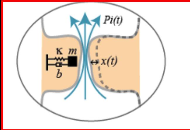
$$\left\{ \begin{aligned} \frac{dx}{dt} &= y, \\ \frac{dy}{dt} &= (1/m) \left[ -k(x)x - b(y)y - cx^2y + a_{lab}P_s \left( \frac{\Delta a + 2\tau\tau}{a_{01} + x + \tau y} \right) \right]. \end{aligned} \right.$$
