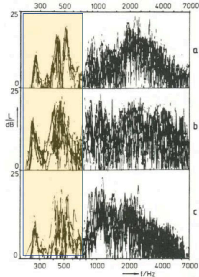
Figure 11: Response Curves of different violins; (a) ten old, distinguished violins; (b) ten violins made by modern craftsmen; (c) ten mass-produced violins.
