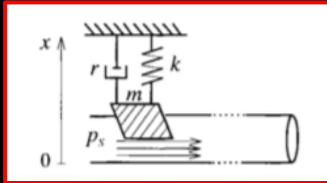
$$\begin{aligned} m\ddot{x} + r\dot{x} + kx &= \gamma(p_s - p(t)) \\ p(t) &= (g * u)(t) \\ u(t) &= \gamma_2 x(t) \sqrt{p_s - p(t)} \end{aligned}$$
