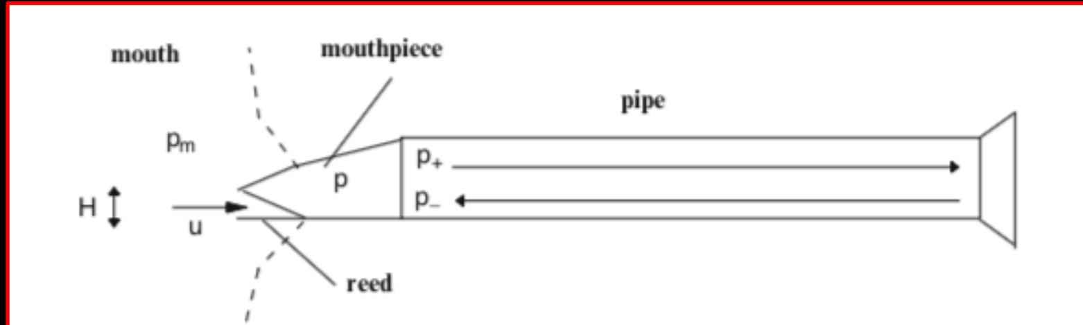
$$\phi = \phi_0 \left(1 - \frac{\Delta p}{p_m}\right) \sqrt{\frac{\Delta p}{p_m}} \quad \text{si. } \Delta p \leq KH_0$$
