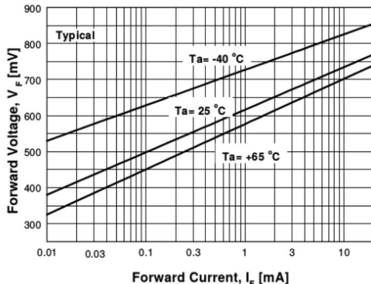
**Figure 6. Forward Voltage vs Ambient Temperature**
