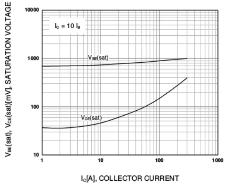
Figure 4. Base-Emitter Saturation Voltage
