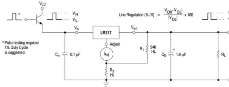
Figure 3. Line Regulation and  $\Delta I_{Adj}$ /Line Test Circuit
