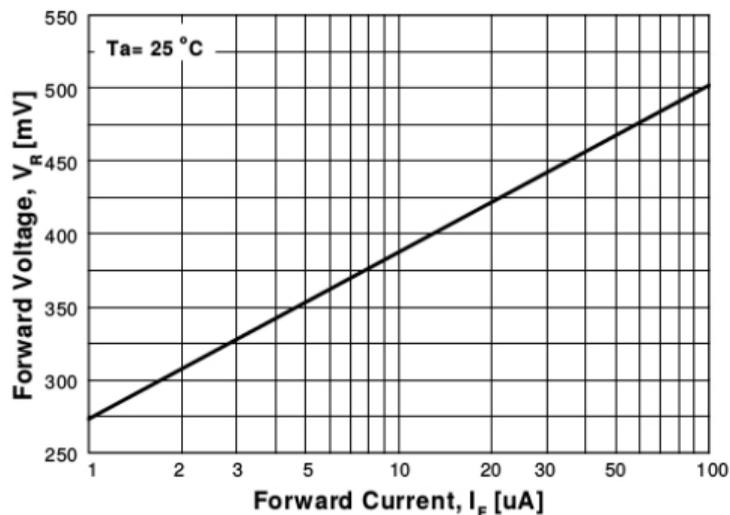
Figure 3. Forward Voltage vs Forward Current
