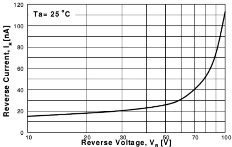
GENERAL RULE: The Reverse Current of a diode will approximately double for every ten (10) Degree C increase in Temperature
