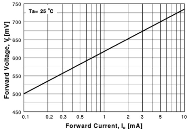
Figure 4. Forward Voltage vs Forward Current
