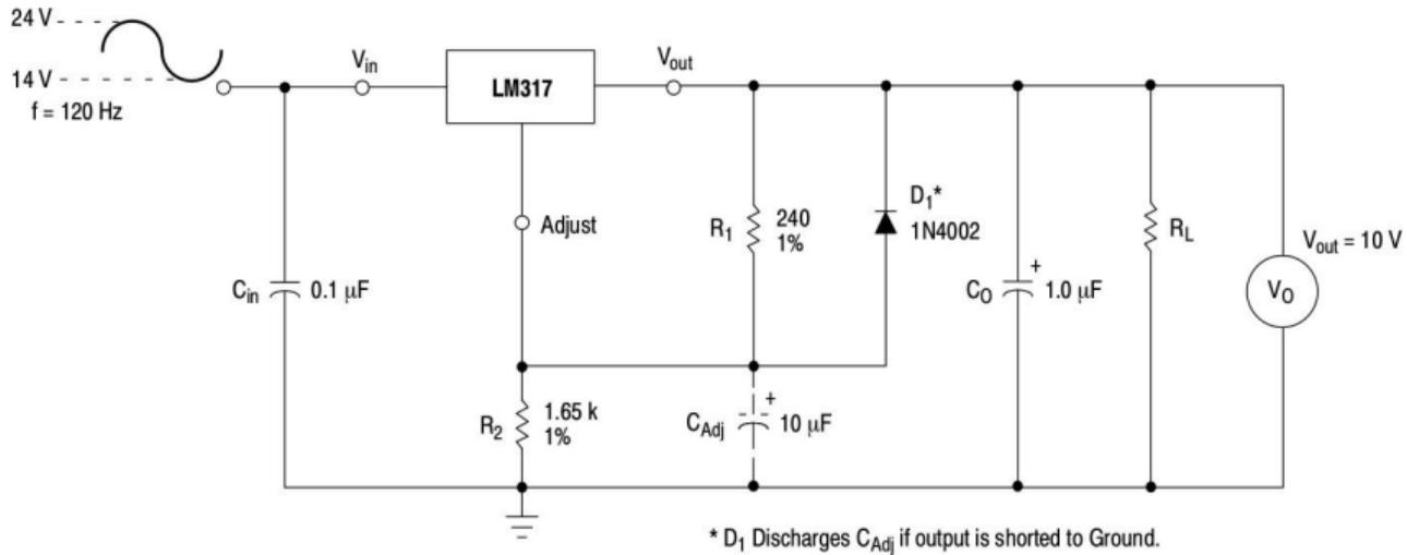
Figure 6. Ripple Rejection Test Circuit
