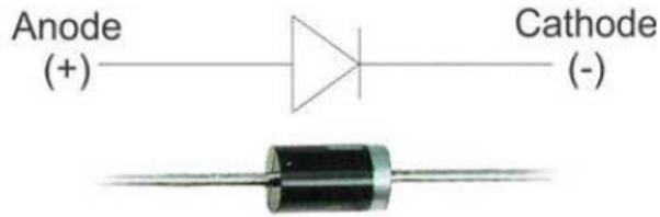
$$I_D(V_D) = I_S \left\{ \exp\left(\frac{q V_D}{\eta K_B T}\right) - 1 \right\}$$
