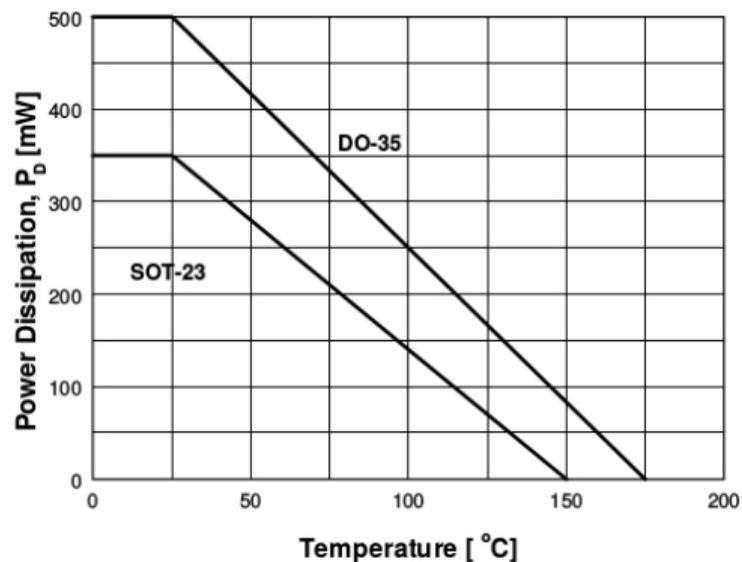
Figure 10. Power Derating Curve
