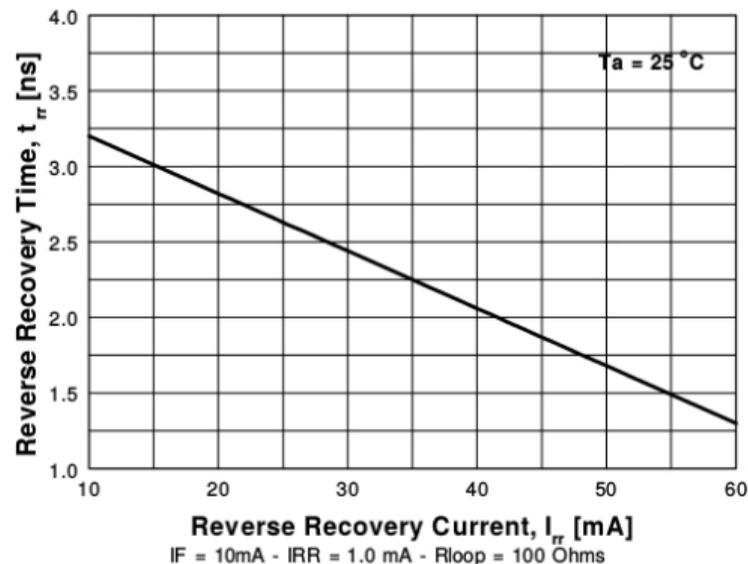
Figure 8. Reverse Recovery Time vs Reverse Recovery Current
