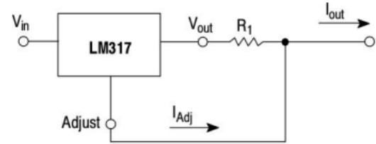
$$\begin{aligned} I_{out} &= \left( \frac{V_{ref}}{R_1} \right) + I_{Adj} \\ &= \frac{1.25 \text{ V}}{R_1} \\ 10 \text{ mA} &\leq I_{out} \leq 1.5 \text{ A} \end{aligned}$$
