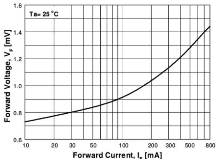
**Figure 5. Forward Voltage vs Forward Current**
