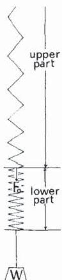
Fig. 2. The division of the spring into two parts to demonstrate the equivalence of Eqs. (2a) and (2b).
