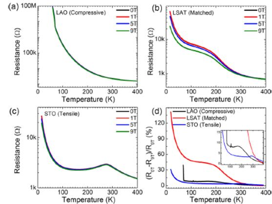
FIG. 2. Resistance as a function of temperature loops under increasing out-of-plane magnetic fields for (a) compressively strained film on LAO, (b) lattice matched film on LSAT, and (c) tensile strained film on STO. (d) MR at 9T for each of the three films.
