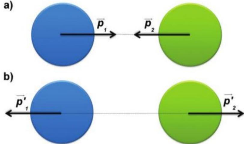
$$\vec{P} = cte = \underbrace{\vec{P}_1^0 + \vec{P}_2^0}_{\vec{P}_1 + \vec{P}_2} = \vec{P}_1 + \vec{P}_2$$
