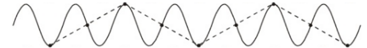
b) Aliasing caused by sampling at less than the Nyquist sampling rate
