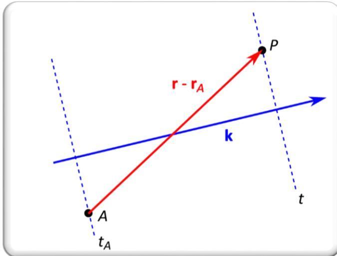
$$t = t_A + \frac{\vec{k} \cdot (\vec{r} - \vec{r}_A)}{\omega} \quad \xrightarrow{\vec{k} = k\hat{k}} \quad t = t_A + \frac{\hat{k} \cdot (\vec{r} - \vec{r}_A)}{c_s}$$
