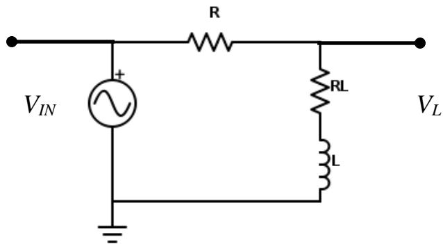
$$V_L = I * (R_L + j\omega L) \quad R_T = R_L + R$$
