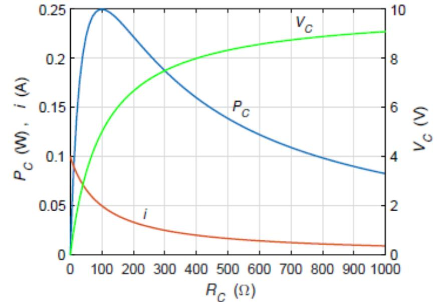
$$V_{th} = 10 \text{ V} \quad R_{th} = 100 \Omega$$
