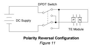
conditions that can occur when mode changes are made, otherwise you may create damaging shortcircuits across your power supply. In automatic controls, a suitable 'deadband' for triggering mode changes is also recommended to prevent 'chattering' (i.e., high frequency toggling between modes).
