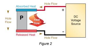
practical TE devices (as will be explained in the next question). While the illustration here—for simplicity's sake—shows 'hole' flow through the connections to the power supply, in reality, electrons are the charge carriers through the copper pathways.
