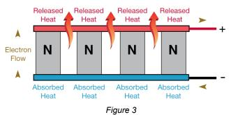
semiconductor pellet is rated for only a very small voltage—as little as tens of millivolts—while it can draw a substantial amount of current. For example, a single pellet in an ordinary TE device might draw five amps or more with only 60 mV applied; if wired in parallel in a typical 254-pellet configuration, the device would draw over 1270 amps with the application of that 60 mV (assuming that the power supply could deliver that much current).
