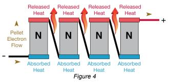
the desired electrical and thermal configuration while better optimizing the thermoelectric effect.
