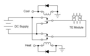
Figure 12: DPDT-Center-Off Simulation
