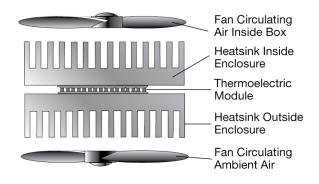
Figure 8: Conceptual Drawing of Air-to-Air Thermoelectric Cooling System
